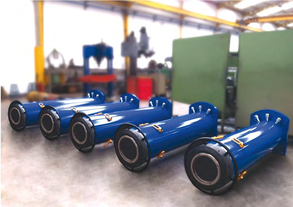
Double acting 605 Ton cylinders with lock nut. Stroke: 1.300mm.
