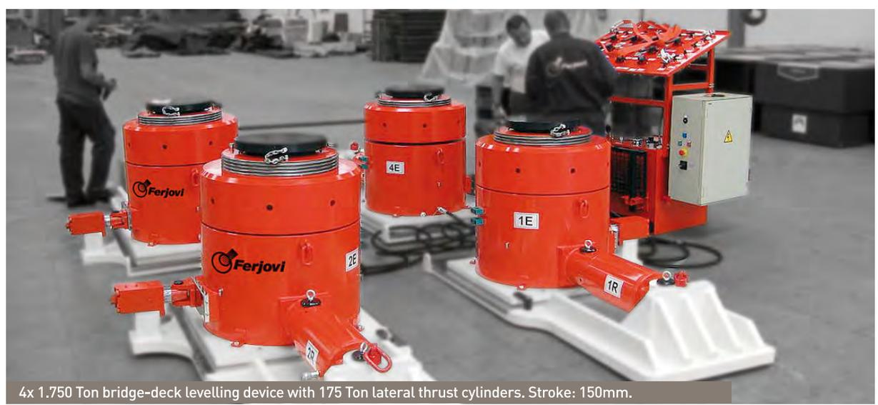
4x 1.750 Ton bridge-deck levelling device with 175 Ton lateral thrust cylinders. Stroke: 150mm.
